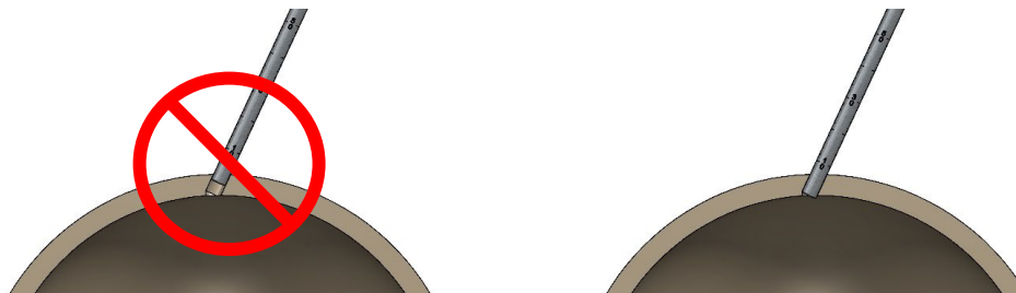
Figure 8: Incomplete Drilling (left); Clearance Mandrel with Complete Drilling (right)
