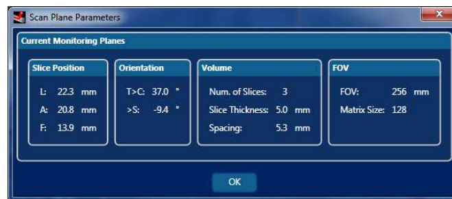
Figure 8.8.2: Scan Plane Parameters for Siemens or IMRIS MRI
