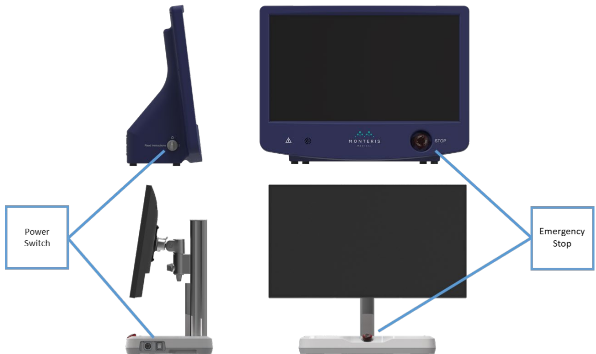
Figure 7.4: Control Workstation Gen 3 (top); Control Workstation Gen 4 (bottom)
