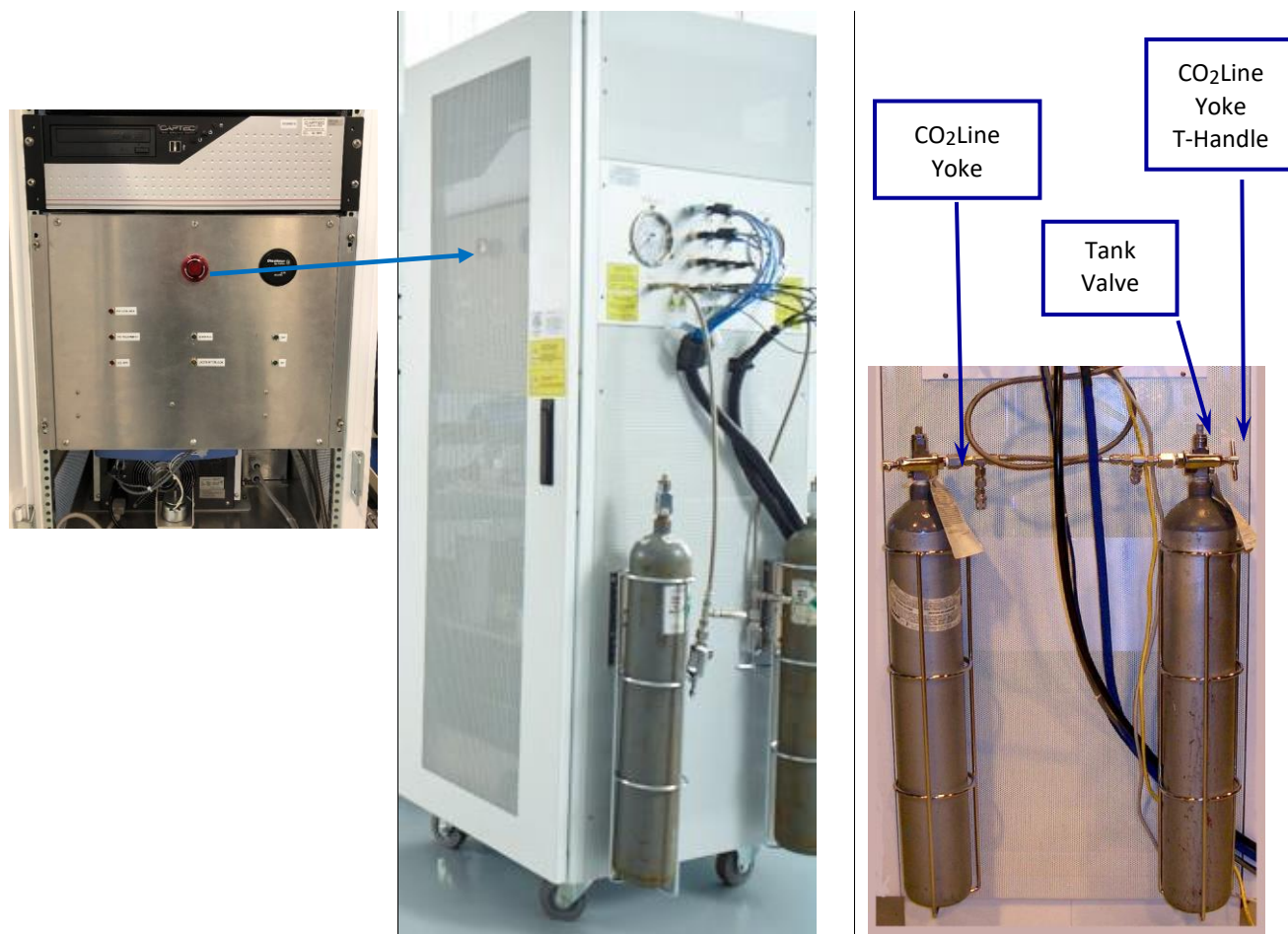
Figure 7.2 Emergency Stop and Electronics Rack with mounted CO 2 Tanks
