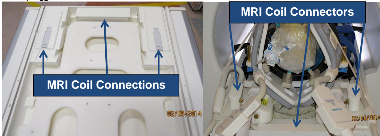
Figure 8.4: MR Coil Connections for Siemens Aera and Skyra MRI
