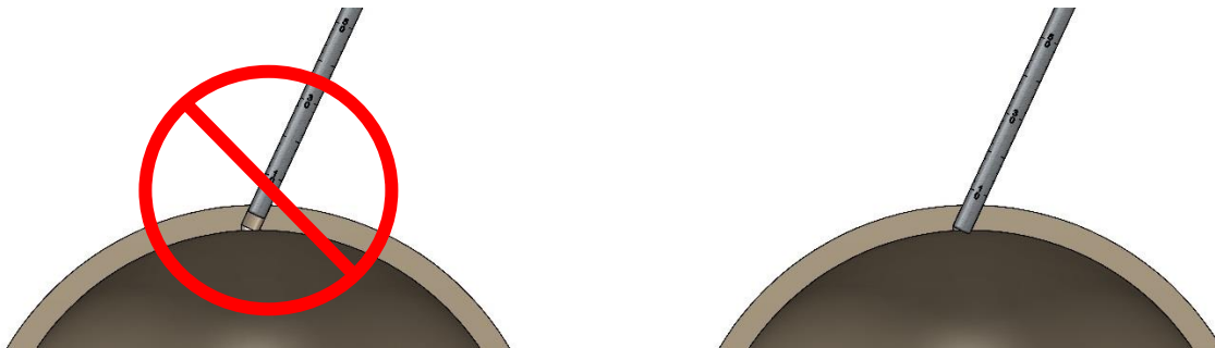
Figure 7: Incomplete Drilling (left); Clearance Mandrel with Complete Drilling (right)
