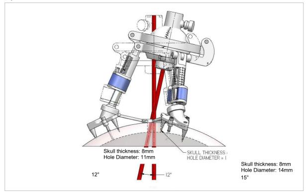
Figure 6: Adjustability for 11 mm (left) and 14 mm (right) Pre-Drilled Holes through Skull
