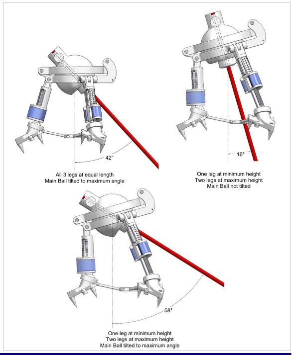
Figure 5: Adjustability when there is not a pre-drilled access in skull.
