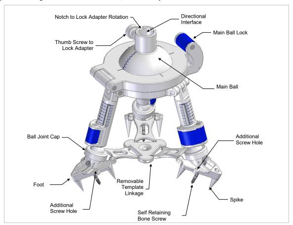
Figure 1: Diagram of AXiiiS illustrating the device's main functional parts.
