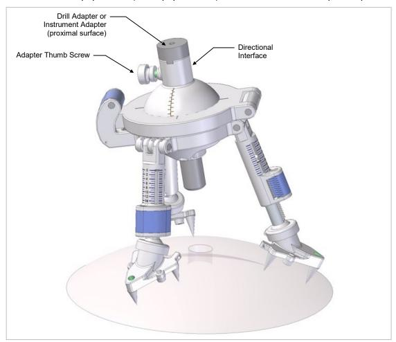
Figure 8: Illustration of the mounting of an accessory Instrument Adapter to the AXiiiS.
