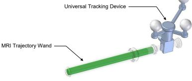
Figure 7.1: Illustration of IGS Universal Tracking Device attached to MRI Trajectory Wand.
