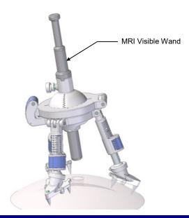
Figure 7: Illustration of MRI Trajectory Wand mounted in the AXiiiS.
