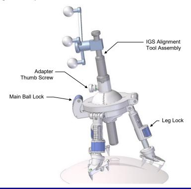
Figure 7.2: Illustration of the MRI Wand (with IGS Tracking) attached to the AXiiiS.
