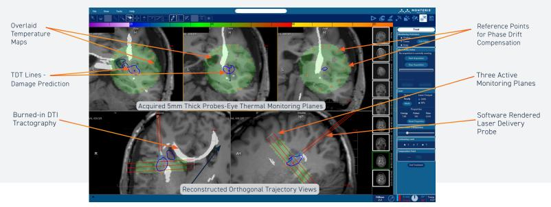
\*"Voxel" is a three dimensional pixel obtained by a LITT system from the MR thermometry which, when combined, creates an enhanced visualization of the ablation zone.
